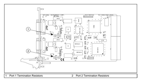
Figure C-5. Location of Termination Resistors on a PXI-8460
