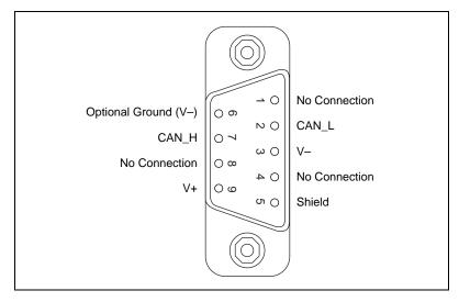
Figure C-1. Pinout for 9-Pin D-Sub Connector
