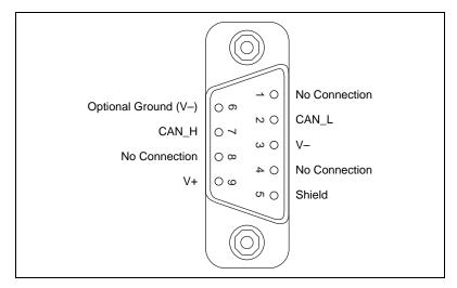
Figure B-1. Pinout for 9-Pin D-Sub Connector
