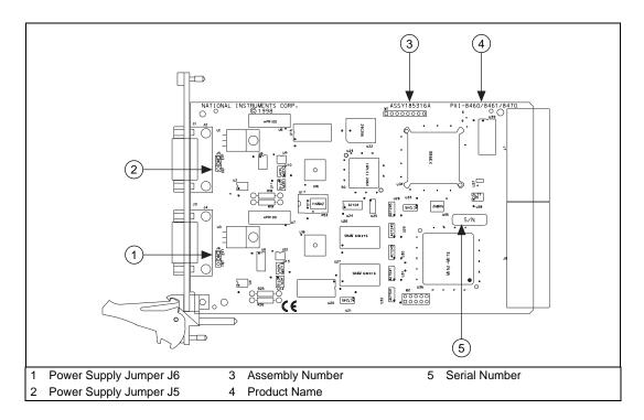
Figure B-3. PXI-8461 Parts Locator Diagram
