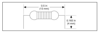
Figure C-6. Preparing Lead Wires of Replacement Resistors
