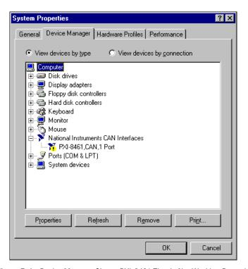
Figure D-1. Device Manager Shows PXI-8461 That Is Not Working Properly
